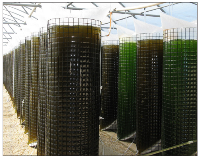
Figure 11. Polyethylene bags used for continuous culture of microalgae. Bags are sealed top and bottom; one port in the bag introduces sterile medium and the other is used to harvest microalgae. The bags are supported by a cylindrical, steel mesh frame coated with vinyl (courtesy Bay Shellfish, Tampa, FL).
